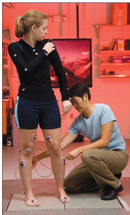
Biomedical engineer Lena Ting (right) prepares to measure how a volunteer's muscles react when her balance is disturbed by a moving platform. Courtesy of Georgia Institute of Technology.
