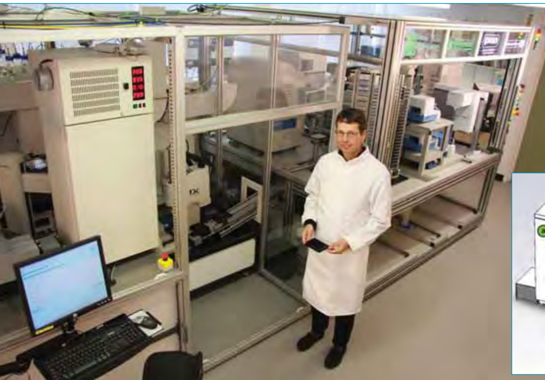
ADAM is a 5-meter-long robot whose equipment includes cameras, sensors, and computers in addition to (a) an automated -20°C freezer, (b) three liquid handlers, (c) three automated +30°C incubators, (d) two automated plate readers, (e) three robot arms, (f) two automated plate slides, (g) an
