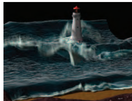
Oscar-winning Water. A 2008 Academy Award for Science and Engineering went to developers of a fluid simulation system used in a number of movies produced by Industrial Light & Magic. As shown here, the Oscar-winning program generates realistic-looking waves and splashes using the particle level set method and an additional method that simulates how the spray interacts with itself and the surrounding water. Courtesy of Ron Fedkiw
