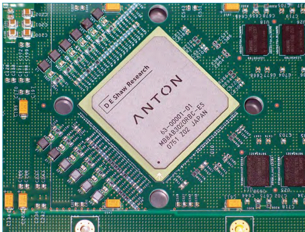
Anton is designed for a specific task: molecular dynamics simulations. Here is one of the first Anton application-specific integrated circuits (ASIC), which arrived in January 2008. Reprinted from Anton, a special-purpose machine for molecular dynamics simulation, David E. Shaw, et al., Communications of the ACM 51:91-97 (2008) with permission from the ACM.
