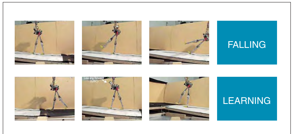
On its first try at a slope, Runbot teeters backward and falls (top). But it learns from its mistakes: On subsequent efforts, Runbot makes it to the top of the hill (bottom). Courtesy of Florentin Wörgötter.
