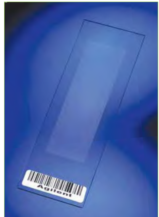
Left: The oligonucleotide array (such as the GeneChip from Affymetrix) uses probes that are short strands of DNA synthesized directly on the chip, and a single type of cell is examined at a time. Courtesy of The Science Creative Quarterly, artist: Jiang Long. Right: InkJet Array. Agilent Technologies, Inc. uses inkjet printing technology to synthesize oligonucleotide probes on a chip. Courtesy of Agilent.
