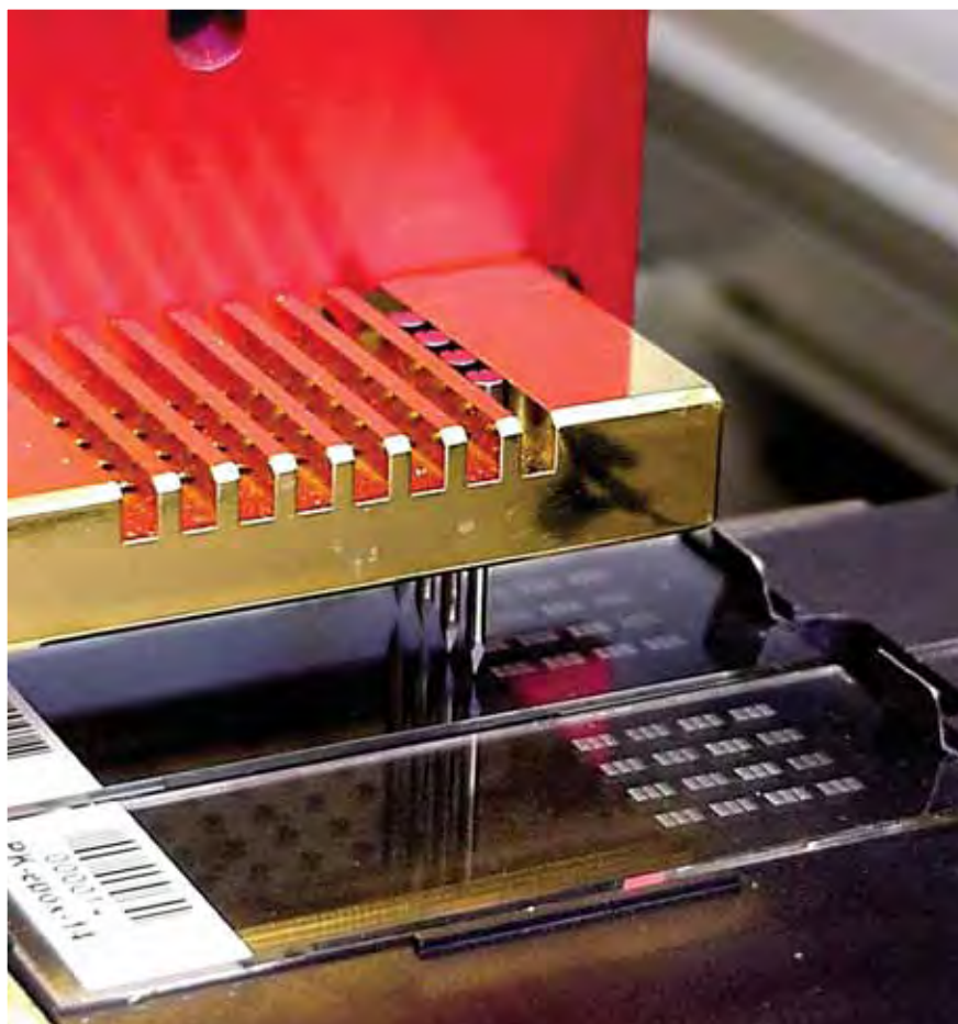
Making of a microarray: A robot spots a glass slide. Courtesy of NIAID Microarray Research Facility.
